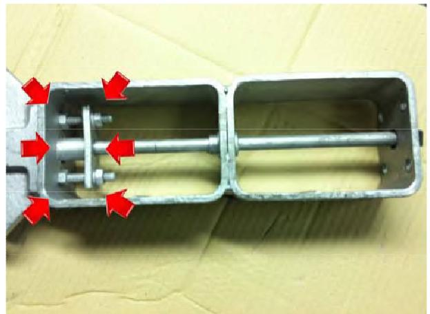
Another important aspect is represented by the choose to have a double bracket on the upper side and a single bracket on the bottom side to mount these valve on the insulated lines without problem.
